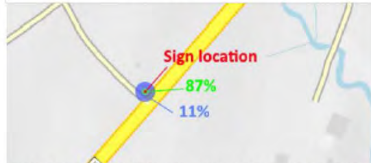
Figure 12 The error distribution of the Vionice detections shown as a percentage plot (top), and visualized on a map (bottom). The map: if a sign is located on the red dot, 87% of the Vionice detections in this dataset would be placed inside the green circle, 11% would be placed inside the blue circle, and the remaining 2% would be outside of the circles.
